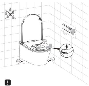
Please cover the spray arm during testing to avoid sprayed Please check for leaks and drips before caulking
