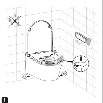
Please cover the spray arm during testing to avoid sprayed Please check for leaks and drips before caulking
